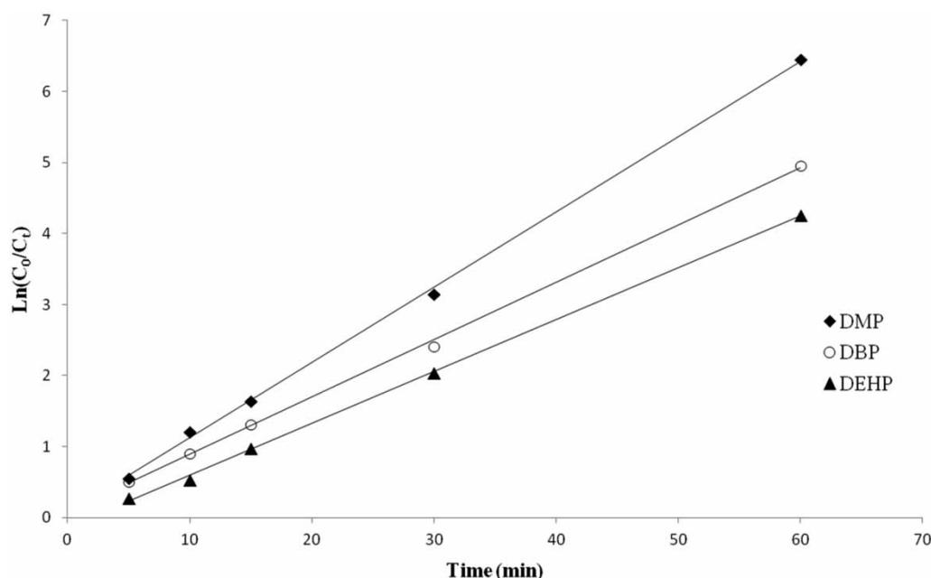
**Figure 5** | Degradation kinetic fitting curves of different phthalic acid esters during UV-Fenton process;  $C_0$ : concentration at time point 0 min,  $C_t$ : concentration at time point t min.
