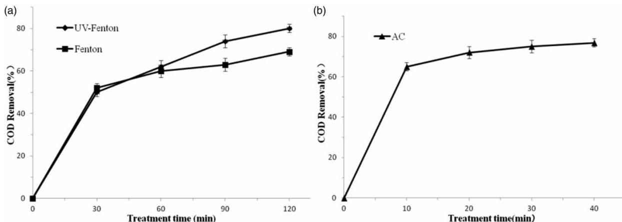
**Figure 1** | Removal rate of COD after UV-Fenton, Fenton or activated carbon adsorption treatment; AC: activated carbon.
