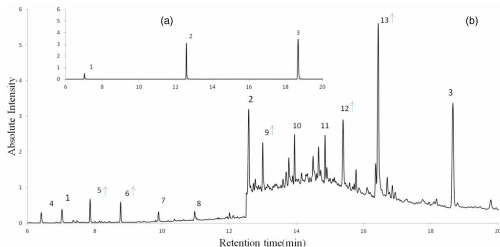
**Figure 6** | Intermediates analysis results tested by total ion current gas chromatogram on GC/MS; (a) Untreated, (b) Treated by UV-Fenton process for 10 min; Peak 1, 2 and 3 represented DMP, DBP, DEHP respectively. Peak 4–13 represented other compounds formed in the UV-Fenton process. The arrows represented peak areas increasing significantly compared with that UV-Fenton treated for 5 min.
