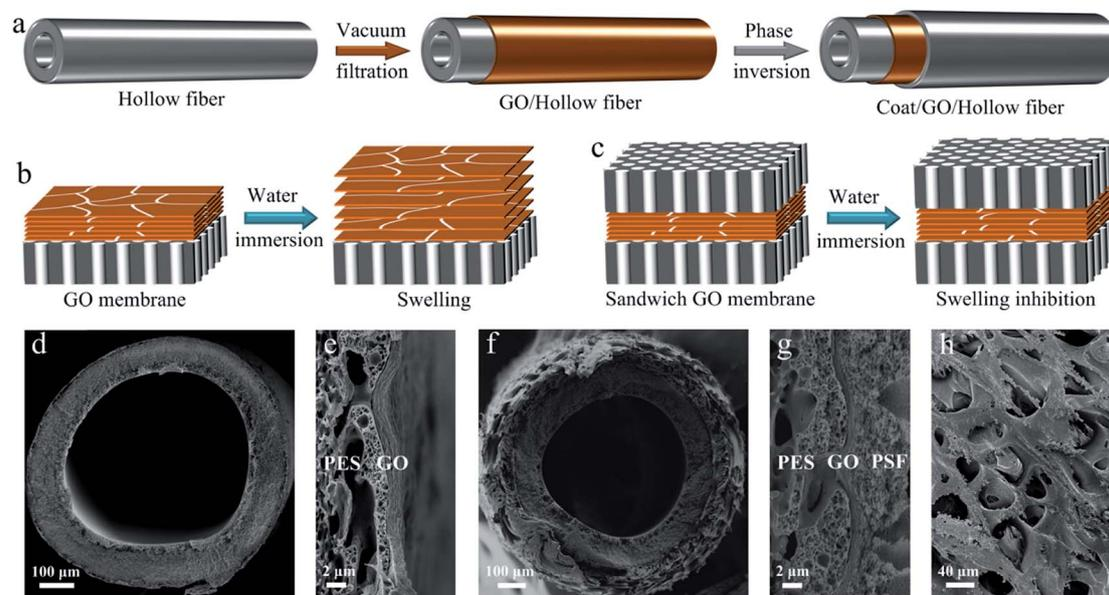
Fig. 1 SGO hollow fiber membranes. (a) The schematic of preparation of SGO hollow fiber membranes. (b and c) The schematics of GO membranes with increased interlayer spacing and SGO membranes with confined interlayer spacing in water. SEM images of (d and e) the GO/PES hollow fiber membrane and (f–h) the SGO-W/PES hollow fiber membrane.
