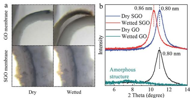
Fig. 2 Swelling properties and interlayer spacing. (a) Optical microscopy images of the dry and 1 h wetted GO/PES and SGO-W/PES hollow fiber membranes. (b) XRD patterns of the dry and 1 h wetted GO/PES and SGO-W/PES hollow fiber membranes.
