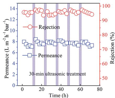
Fig. 4 Long-term stability of the SGO-W/PES membrane at 2.0 bar. The separation performance showed a small fluctuation over 3 days and ultrasonic treatment five times.
