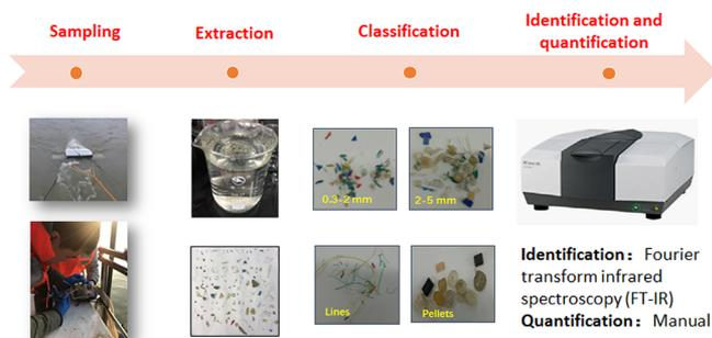
**Figure 1.** Flowchart depicting the full process for microplastic analysis used in the present study, including sampling, extraction, classification and identification, and quantification.
