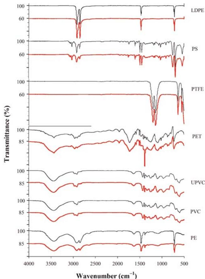
**FIGURE 3:** Fourier transform infrared spectroscopy spectra of tested polymers before (black line) and after (red line) digestion. Transmittance for low-density polyethylene, polystyrene, and polytetrafluoroethylene are all the same scale, whereas the rest are a different scale. LDPE = low-density polyethylene; PE = polyethylene; PET = polyethylene terephthalate; PS = polystyrene; PTFE = polytetrafluoroethylene; PVC = polyvinyl chloride; UPVC = unplasticized polyvinyl chloride.
