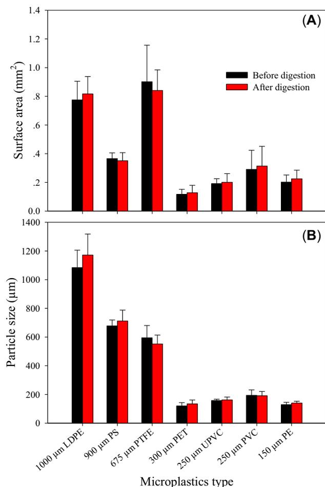
**FIGURE 2:** (A) Surface area and (B) particle size (average  $\pm$  standard deviation) of tested polymers before and after treatment with the present method ( $t$  test,  $p > 0.05$ ). LDPE = low-density polyethylene; PE = polyethylene; PET = polyethylene terephthalate; PS = polystyrene; PTFE = polytetrafluoroethylene; PVC = polyvinyl chloride; UPVC = unplasticized polyvinyl chloride.
